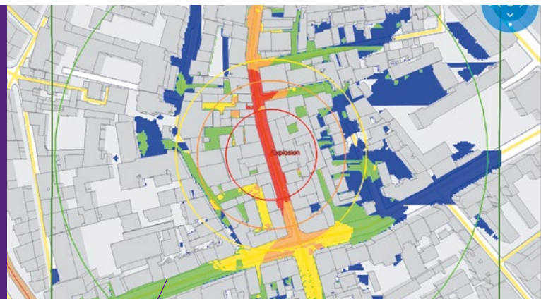
Danger zones from an explosion in a city (fast-running code FLASH) compared to «free-field» circular zones
