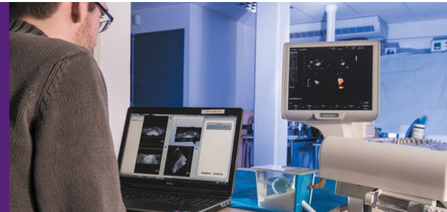
3D ultrasound image-guided robot for prostate cancer treatment (brachytherapy). Development of a clinical version of the system
