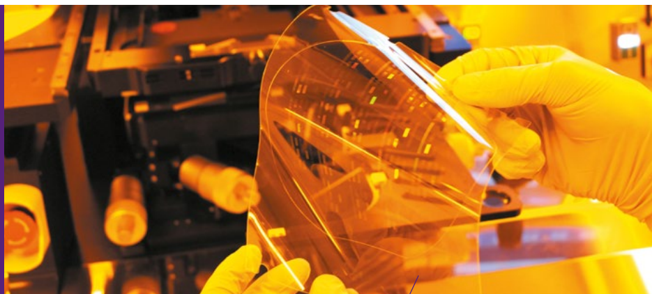
Nano-imprint of cavities for flexible displays
